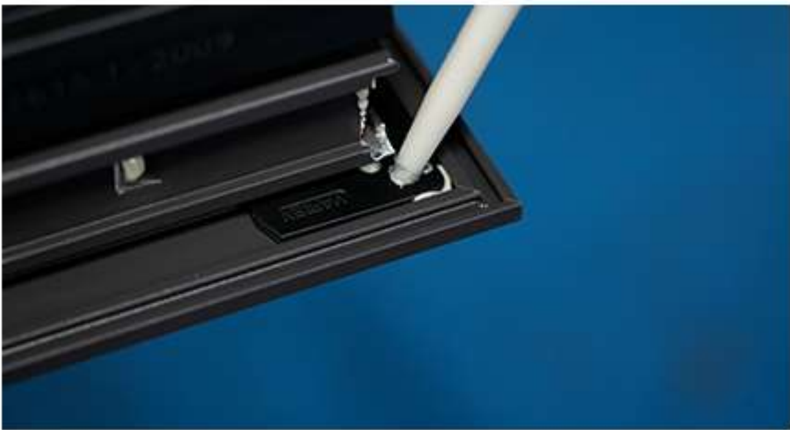
Injection Method for Corner Angle Bonding: German Weiss Cosmofen Duo
